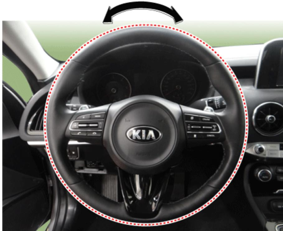
3. If the play exceeds standard value, inspect the steering column, shaft, and linkages.
